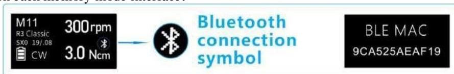
At the same time, the advanced mode setting also provides the MAC address of the Bluetooth function of the device. It is convenient for other devices to identify the physical address when searching the Bluetooth connection of the device.
