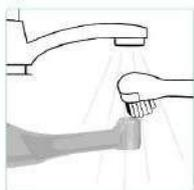
Disconnect the contra angle from the motor hand piece. Clean off the cutting, Debris with running water and a soft brush and then wipe off the water.
