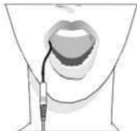
\* M0 is the Apex Locating mode by default. It is necessary to connect the measuring wire with the file clip and the lip hook, and place the lip hook in the corner of the patient's mouth.
