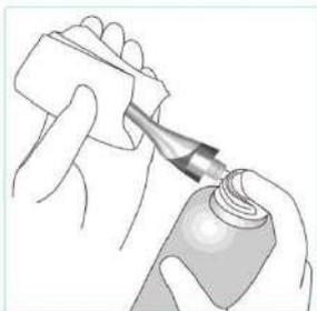
Screw the nozzle onto the spray can. Then insert it into the connection end of the contra angle, and spray for 2s. Using gauze etc to wipe excess spray off the outside of the contra angle.
